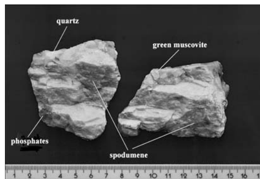
Photo 2. Massive spodumene aggregates, associated with quartz, green muscovite and Li, Mn, Fe phosphates.
